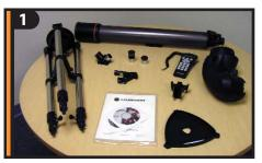
Your NexStar 80SLT includes: optical tube; fork arm; pre-assembled tripod; computerized hand control; hand control holder; star diagonal; two eyepieces; finderscope; accessory tray; documentation including an owner's manual, The Sky<sup>®</sup> CD and NSOL Telescope Control Software.
